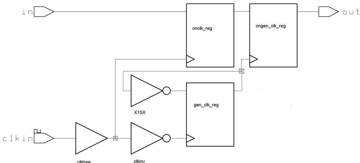
If we ignore the inverter `clkinv` in the path to the clock divider flop `gen_clk_reg`, this circuit is very like the one encountered earlier that had the divide-by-2 outgoing clock. You do a `create_clock` on `clkin`, and a `create_generated_clock` on `gen_clk_reg/Q`, and off you go.
