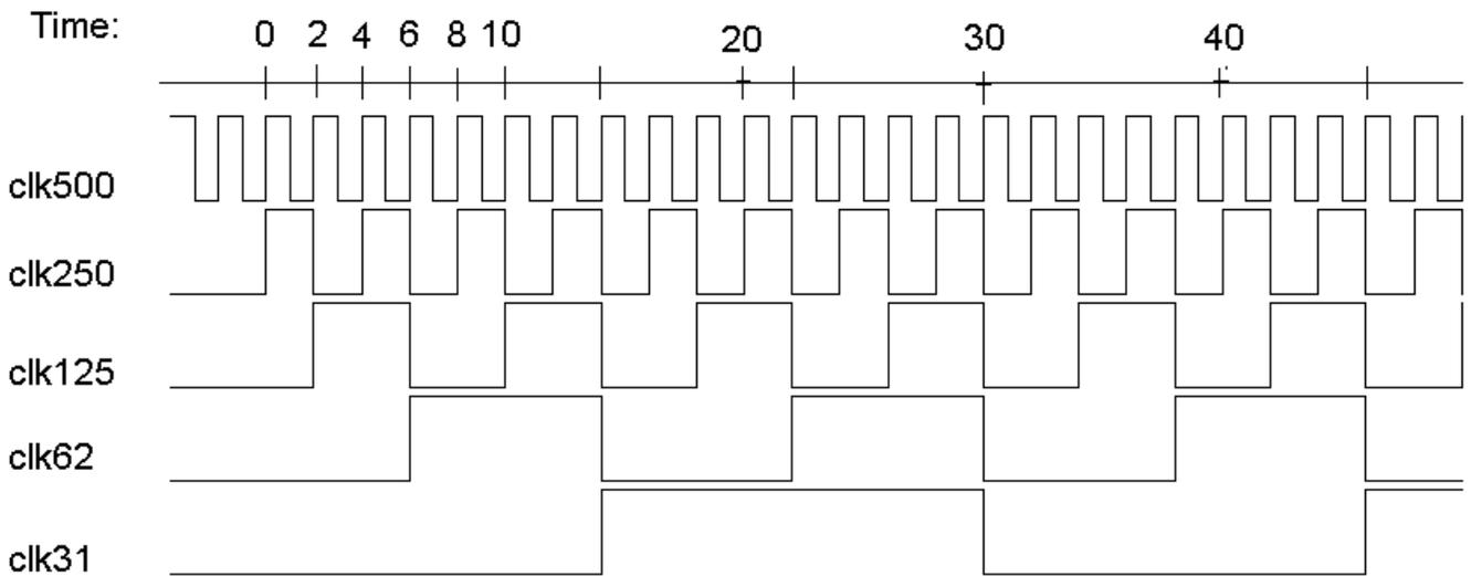
Notice that each clock's rising transition occurs at the falling transition of its parent clock. No two rising edges happen at the same time. This splits the available clock period evenly between setup and hold when transferring data between clock domains.
